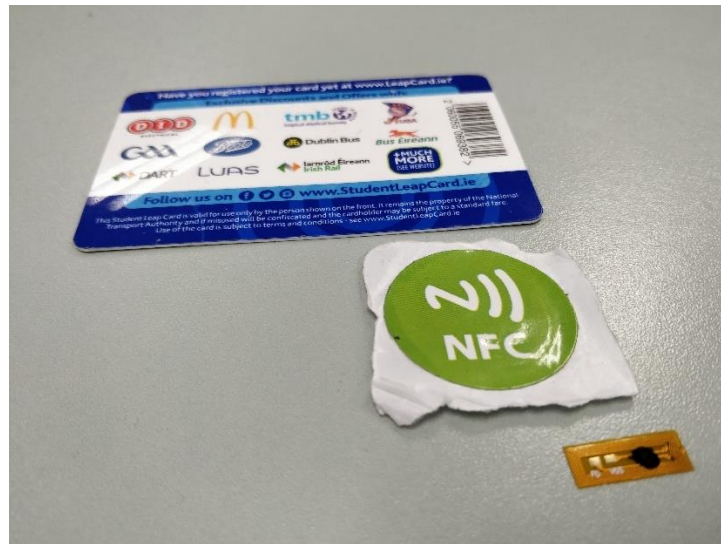
Figure 30 - NFC Tags of Different Shape and Size
